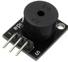
*Fig 8.* Buzzer-ARDUINO (Mishra & Durgaprasad, 2016)
